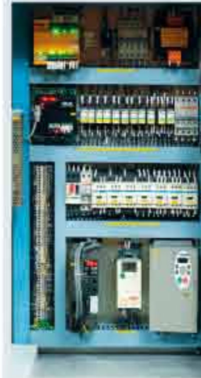
Main electrical components including low voltage components and inverter from Schneider Telemecanique. Main motor and convey belt motor is driven by inverter for stepless speed adjustment.
